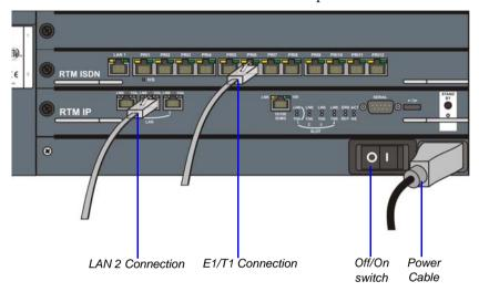
Figure 1-4 RMX 2000 Rear Panel View with Cables
